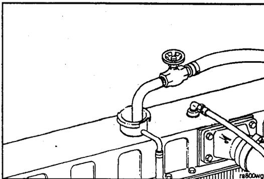
Fill the cooling system with clean water to flush the cooling system.
