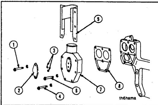
**NOTE:** Do not tighten the capscrews until assembly is complete.
