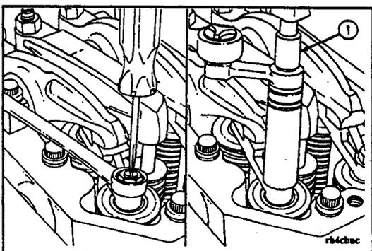
Hold the adjusting screw in this position. The adjusting screw **must not** turn when the lock nut is tightened to its torque value. Tighten the lock nut. The following torque values are given with and without Part No. ST-669 Torque Wrench Adapter (1):
