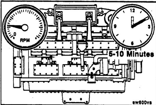
Operate the engine at high idle for 5 minutes (in retard timing mode). This will allow all of the oil to pump out of the injector tappets so a correct injector adjustment can be made.
