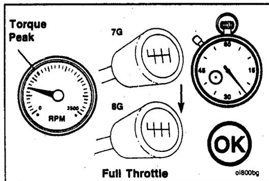
Operation of the engine below peak torque RPM can occur during gear shifting due to the difference of ratios between transmission gears, but engine operation **must not** be sustained more than 30 seconds at full throttle below peak torque RPM.
