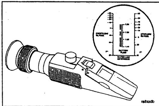
Use the Fleetguard® refractometer, Part No. CC-2800, to check the condition of the battery.
