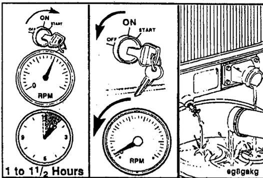
Operate the engine at normal operating temperatures (at least 85°C [185°F]) for 1 to 1 1/2 hours.
