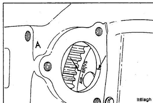
For valve and injector adjustment marks on the flywheel with the engine barring device located on the **left** bank:
