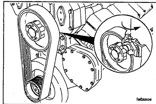
On engines that use a two pulley drive with a 28 inch fan center distance, loosen the bolts that pass through the slotted holes and fan hub bracket of the 28 inch fan center system. The adjusting screw (16) is below the fan hub. The lock nut (17) must be loosened before loosening the fan hub adjusting screw.
