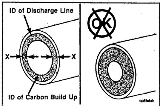
If the total carbon deposit exceeds specifications, continue checking the air discharge line connections, up to the first tank, until total carbon deposit is less than 2 mm [1/16 inch]. Clean or replace any lines or connections that exceed this specification.
