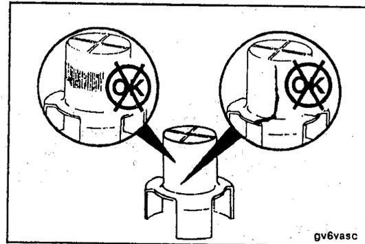
Visually inspect the unloader valves for carbon buildup. If carbon or heavy varnish is present, remove, clean, and inspect the compressor head and the valve assembly. Replace the parts as necessary. Refer to the appropriate Air Equipment Manual listed below for procedures, or contact your nearest Cummins Authorized Repair Location:
