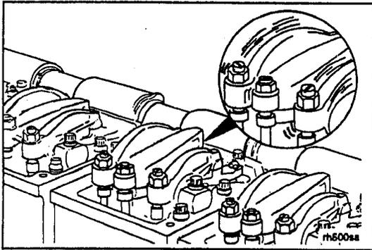
If the rocker levers have **not** been removed, wiggle the valve rocker levers on the two cylinders in question. The crossheads and valves on the cylinder where both levers feel loose are ready to adjust.
