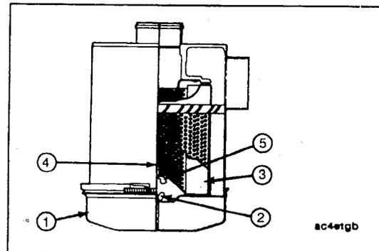
Remove the wing nut (1) that secures the bottom cover (2) to the cleaner housing (3). Remove the cover.
