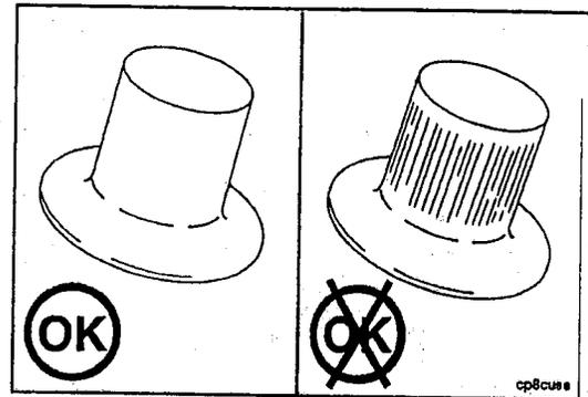
Visually inspect the unloader valves for deep scratches or cracks. Replace if scratched or cracked.
