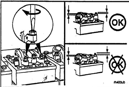
The push rods will be close to the same height above the top of the rocker lever housing on the cylinder ready for valve adjustment.
