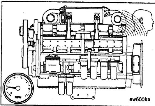
When operating in the advanced mode, a light ticking noise can be noted at the overhead. This sound is normal, and is caused by the actuation of the STC hydraulic tappets during each injection cycle.
