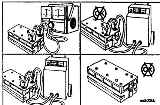
Use battery tester, Part No. 3377193, to test the state-of-charge of maintenance-free batteries.
