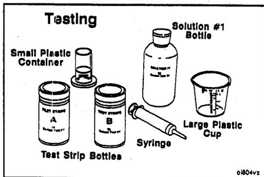
**Testing SCA Concentration Level CC-2626 Test Kit**
