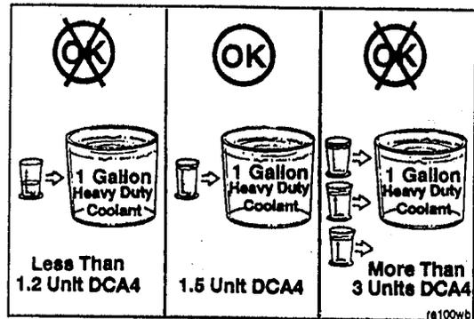
Use the correct Fleetguard® coolant filter to maintain the recommended DCA4 concentration in the system.
