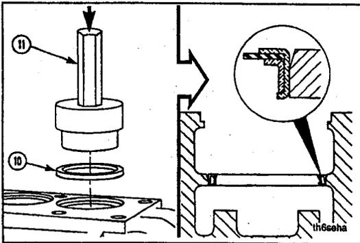
The seal must be installed with the part number positioned up.
