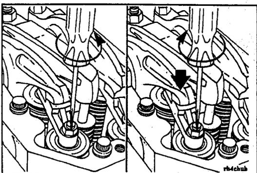
Use the following procedure to adjust both the intake and the exhaust crossheads.
