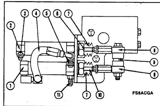
Using your hand, push the throttle lever (9) toward the cylinders (low idle position). The braking cylinder extension rod (10) **must** move smoothly to the retracted position. The cylinder spring **must** push the throttle lever from the air cylinders approximately 1/2 of the distance between the **Idle** and **full fuel** positions.
