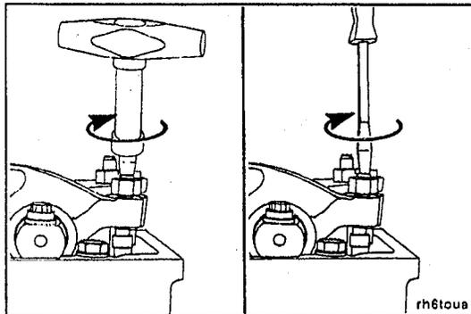
The adjusting screw **must not** turn when the locknut is tightened.
