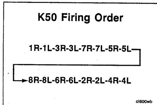
Direction of normal rotation for K38 and K50 engines is **clockwise** when viewing the **front** of the engine.
