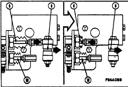
Use your hand, pull the throttle lever (9) away from the air cylinder (full fuel position). Pull the throttle cylinder extension rod (6) toward the throttle lever. The extension rod cap **must** touch the roller tappet on the throttle lever. Release the throttle cylinder extension rod. The rod **must** move toward the cylinder.
