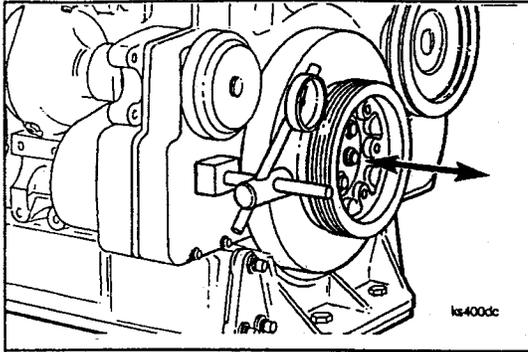
The check can be made by attaching an indicator to rest against the damper or pulley, while prying against the front cover and inner part of the pulley or damper. End clearance **must** be present with the engine mounted in the unit and assembled to the transmission or converter.
