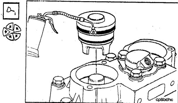
Install the unloading valve body.
