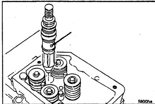
Position the standard injector in the bore. Turn the injector so that the injector screen points toward the hold down capscrew hole on the intake side of the head.
