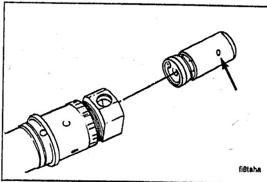
**NOTE:** Do not push the injector on the seat until it is correctly aligned.
