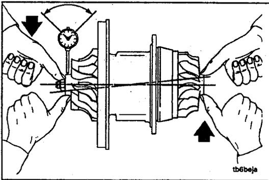
**NOTE:** The compressor and turbine casings do not require removal to measure the radial clearance. The parts are shown removed for clarity.
