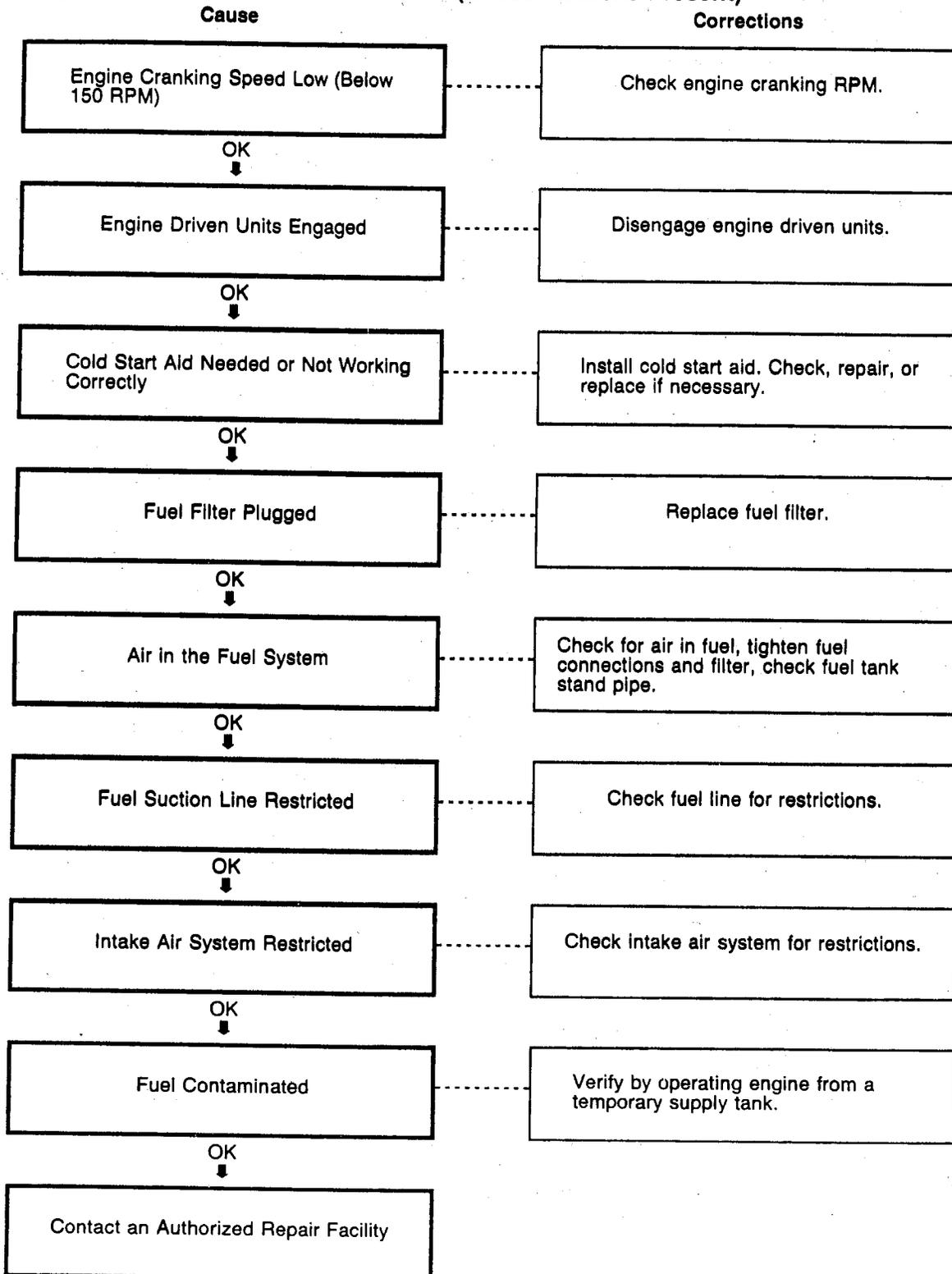
**Engine Cranks But Will Not Start (No Smoke From Exhaust)**
