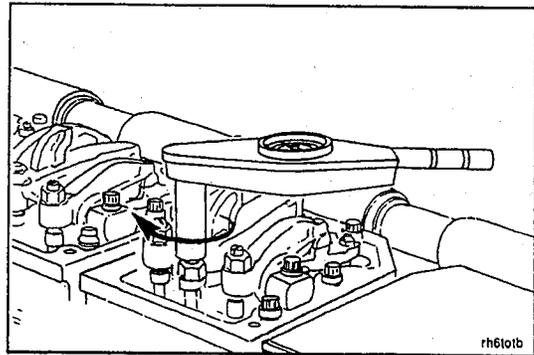
Tighten the adjusting screw to 11 N•m [100 in-lb] to make sure the parts are in alignment and to squeeze the oil out of the valve train.
