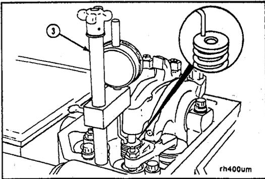
**PT Injector (type D) - Adjustment**
