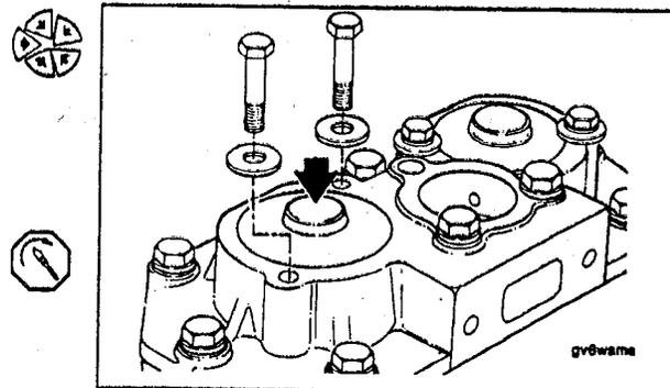
Install the air governor or air governor signal line to the unloader body.
