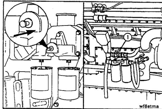
Use engine oil and lubricate the seal on the new filter.
