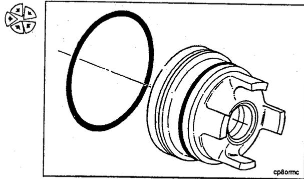
Use clean engine oil to lubricate the seals.
