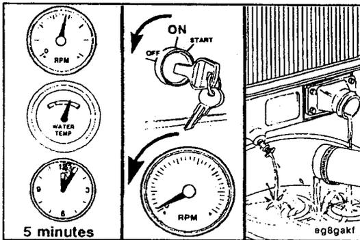
Operate the engine at high idle for 5 minutes with the coolant temperature above 85°C [185°F].
