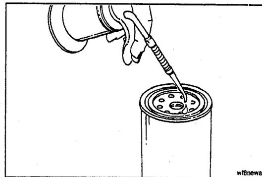
Install the new coolant filter. Turn the filter until the seal touches the filter head. Turn the filter an additional 1/2 to 3/4 of a turn after contact.
