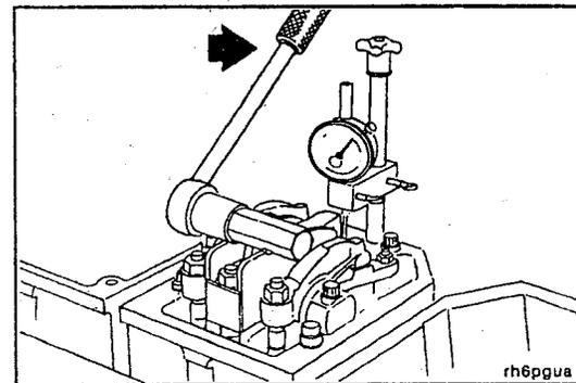
2. Allow the rocker lever to return slowly. Check the injector setting. Repeat the adjustment process if it is not within specification.
