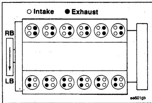
**Intake and Exhaust Valve locations.**
