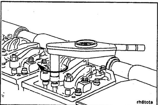
If the barring device was used, allow the spring to push the shaft and gear outward to clear the ring gear. Install the clip.
