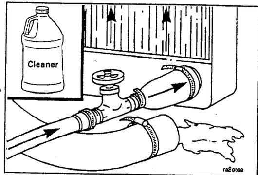
**Warning:** Wait until the temperature is below 50°C [120°F] before removing the coolant system pressure cap. Failure to do so can cause personal injury from heated coolant spray.
