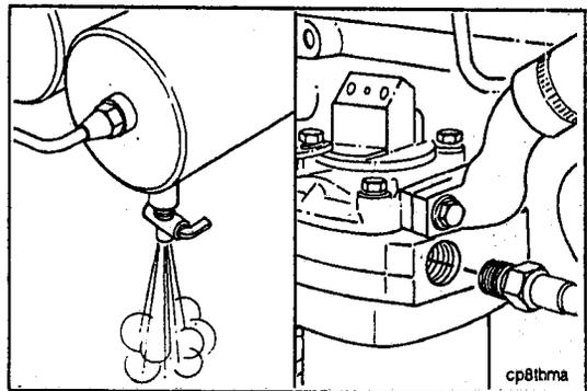
Measure the total carbon deposit thickness inside the air discharge line as shown. If the total carbon deposit (X) exceeds 2 mm [1/6 inch], clean and inspect the cylinder head, the valve assembly, and the discharge line. Replace if necessary. Refer to the appropriate Air Equipment Manual listed below for procedures, or contact your Cummins Authorized Repair Location:
