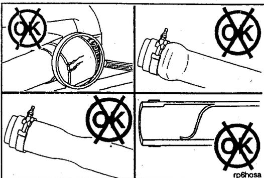
Water line hoses can balloon when a remote, high mounted radiator is used. The maximum permitted radiator height is 18.3 m [60 ft] above the crankshaft centerline.
