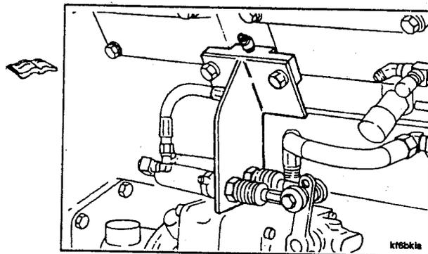
Disconnect the fuel tubing and air hose.
