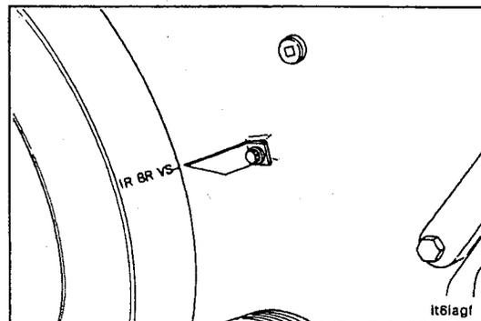
For valve and injector adjustment marks on the flywheel with the engine barring device located on the **right** bank:
