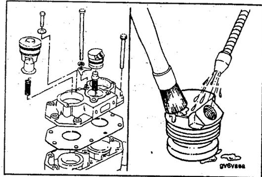
Inspect the upper part of the center unloader valve cap where the rectangular ring seal seats for scoring. Replace if scored.
