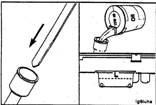
Install the dipstick in the dipstick tube.
