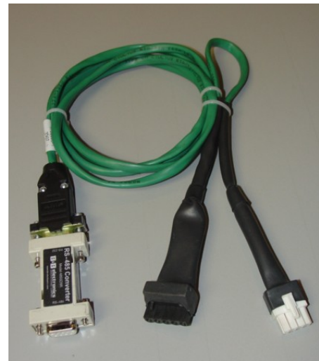
DB9 to 5-pin Connector Service Cable CUMMINS PN 0338-4590
